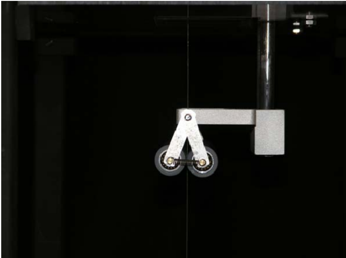
Figure 32. Rollers with new tension spring.
