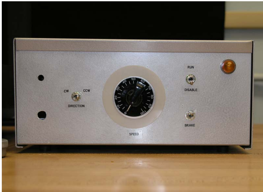
Figure 30. Controller box setup for tachometer output.
